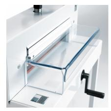
**TRANSPARENT SAFETY GUARD** A cut can only be executed if the hinged safety guard is in the closed position and the blade safety catch is released.
