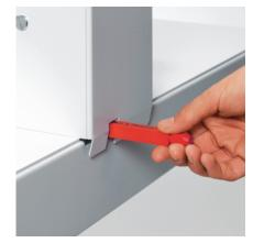
**EASY CUTTING STICK CHANGE** Cutting sticks can be turned or changed easily from the outside of the machine no tools are required.
